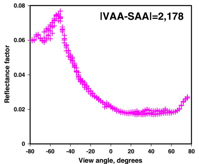
Fig. 2. Red BRF of the Järvelja RAMI stand in the solar principal plane from UAVSpec3 observations on July 27, 2011. All shown BRF observations were retrieved within 2° from the principal plane.
