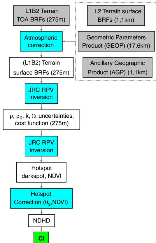
**Fig. 1.** Scheme of clumping index retrieval from MISR data. The gray boxes represent inputs from standard MISR global mode products; the white boxes represent the new high spatial resolution (275 m) products generated in this study; the cyan boxes indicate computational models or codes; and the final green box indicates the result (clumping index). (For interpretation of the references to color in this figure legend, the reader is referred to the web version of this article.)
