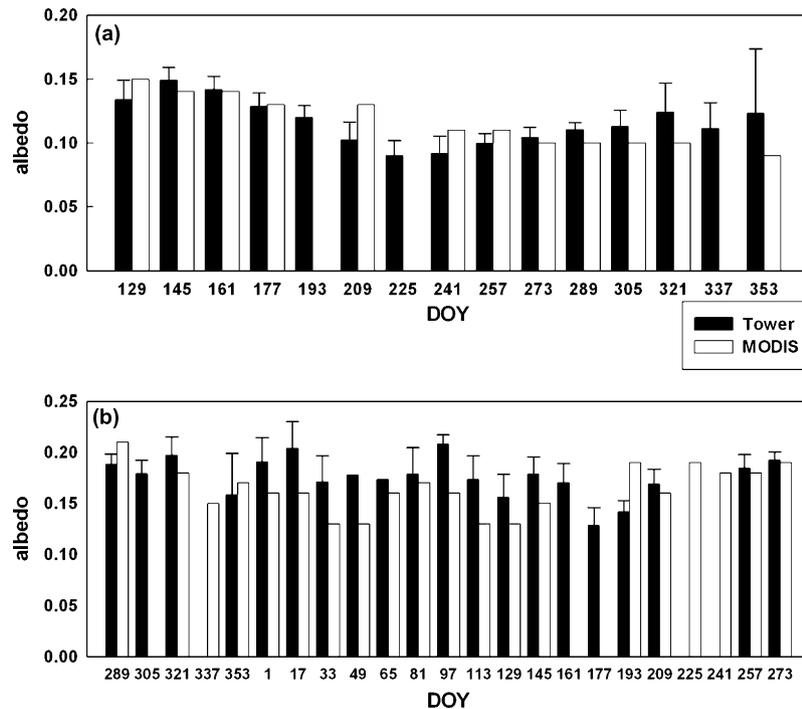
Fig. 5 – Comparison of measured and MODIS derived albedo over (a) the DK site and (b) the FK site. Measured albedos at Terra overpass time were averaged over 16-day in accordance with MODIS albedo product. Error bar means standard deviation for 16-day.
