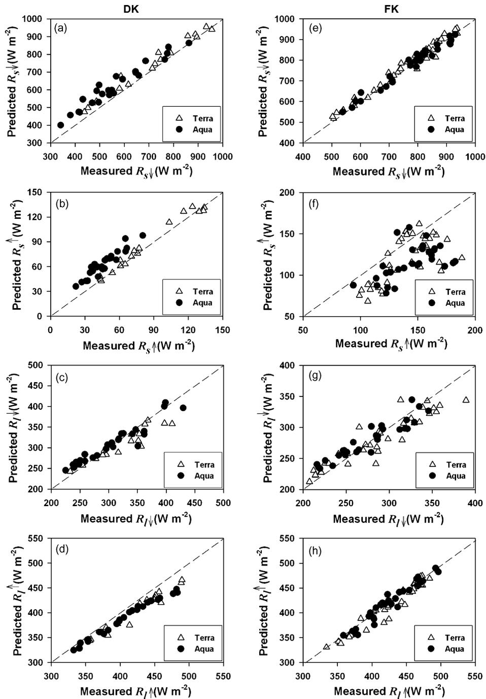
**Fig. 6 – Comparison of measured and MODIS derived four radiation components over the DK and FK sites.  $R_s$  and  $R_l$  are the shortwave and longwave radiation, respectively.  $\uparrow$  and  $\downarrow$  are the upwelling and downwelling streams, respectively. Dash line indicates 1:1 line.**
