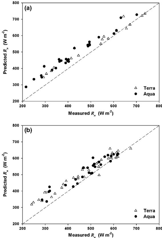
**Fig. 7 – Comparison of measured and MODIS derived net radiation ( $R_n$ ) over (a) the DK site and (b) the FK site. Dash line indicates 1:1 line.**
