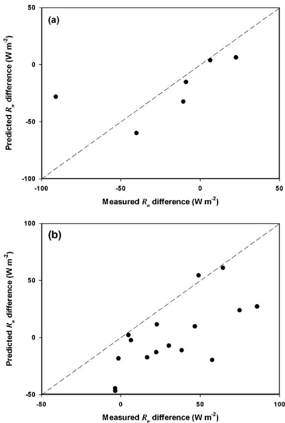
**Fig. 8** – Comparison of measured and MODIS derived net radiation difference (Aqua overpass time minus Terra overpass time) over (a) the DK site and (b) the FK site. Dash line indicates 1:1 line.
