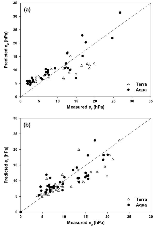
**Fig. 4 – Comparison of measured and MODIS derived actual vapor pressure ( $e_a$ ) over (a) the DK site and (b) the FK site. Dash line indicates 1:1 line.**
